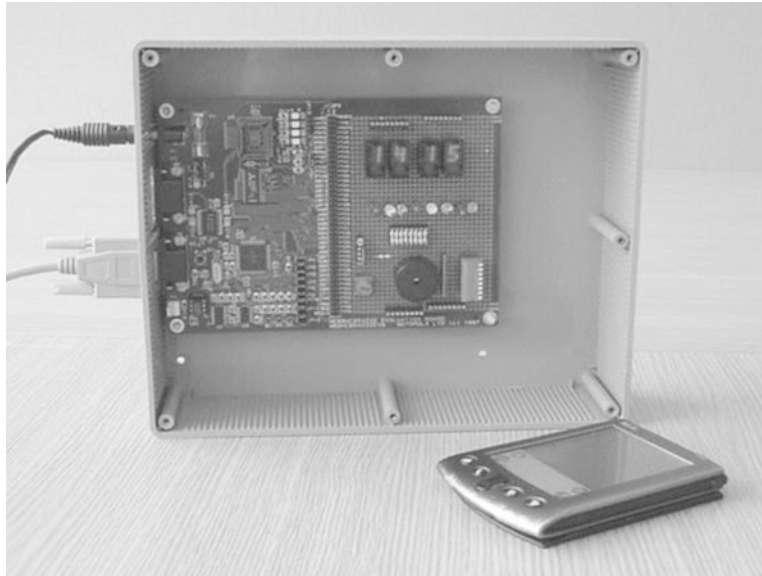
Figure 12.6 A clock display running on the JASPer peripheral box - a PDA is included to give scale
