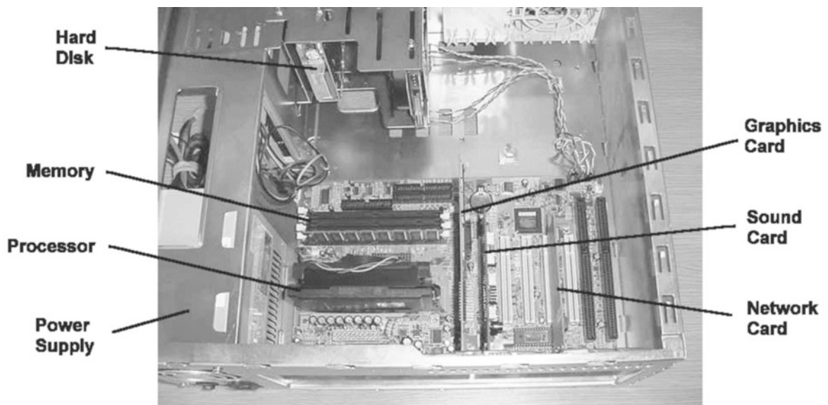
Figure 1.2 The innards of a typical personal computer today
